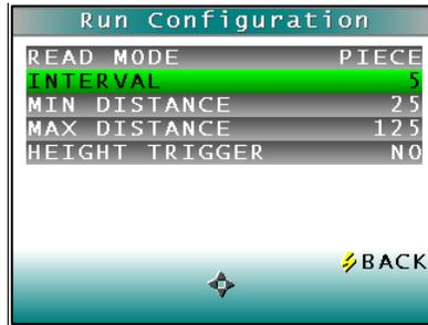
Figure 40. Read Mode Interval
