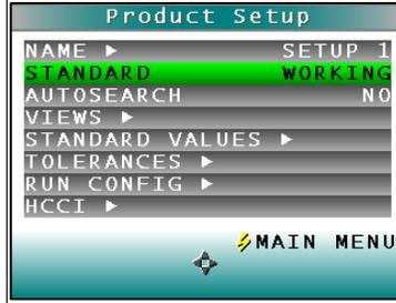
Figure 14. Product Setup > Working Standard Type
