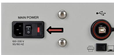
Figure 74 Fuse is located beside I/O rocker switch.
