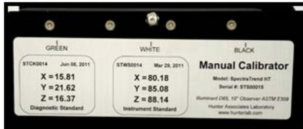
Figure 3. Calibrated Values for the Slide-On Calibrator
