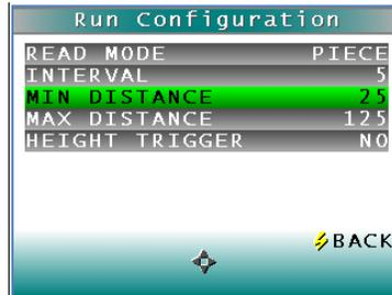
Figure 41. Minimum Height from Belt
