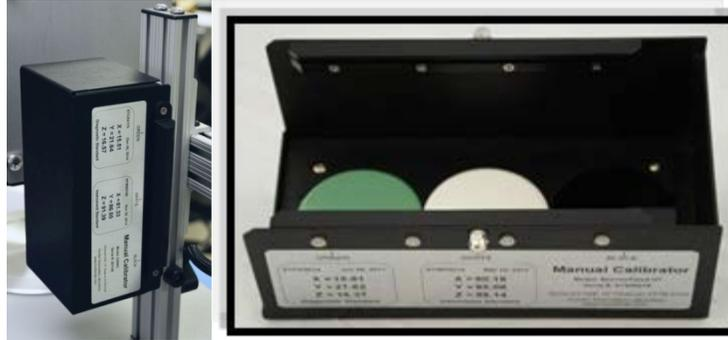
Figure 2. Slide-On Calibrator with storage on stand
